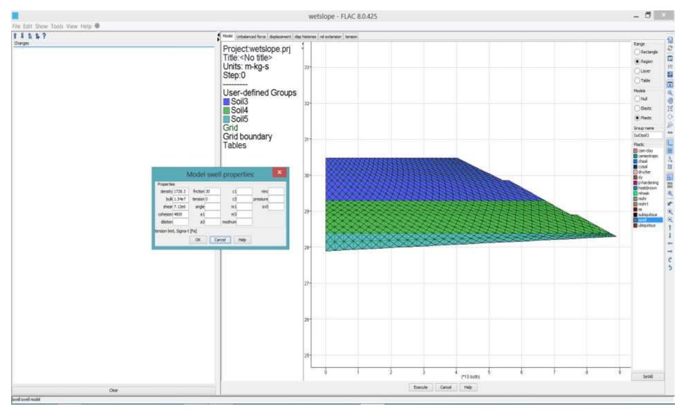
**Step 1-19** Enter the [Material]/[Model], select [Region] range, specify the group name **Soil3** and select the [swell] plastic model. Click the mouse on a zone inside the **Soil3** layer to open the *Model swell properties* dialog. Input the elastic and plastic properties. Leave the swelling properties blank, and the initial behavior will be a Mohr-Coulomb material. Press [OK] to create the *FLAC* command.
