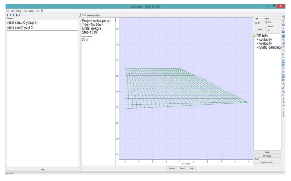
**Step 3-1** Enter the [In Situ]/[Initial] tool and press [Clear? (Displmt&velocity]] to reset displacements and velocities to zero. Press [Execute] to send the commands to *FLAC*.
