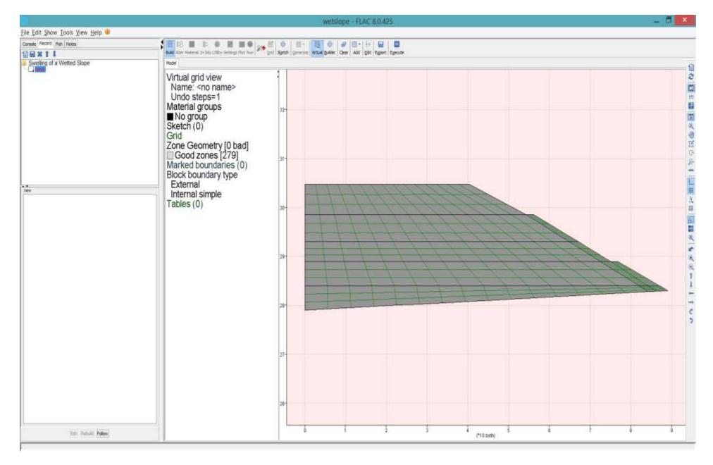
**Step 1-15** Press [Build] and [OK] to create the virtual mesh.
