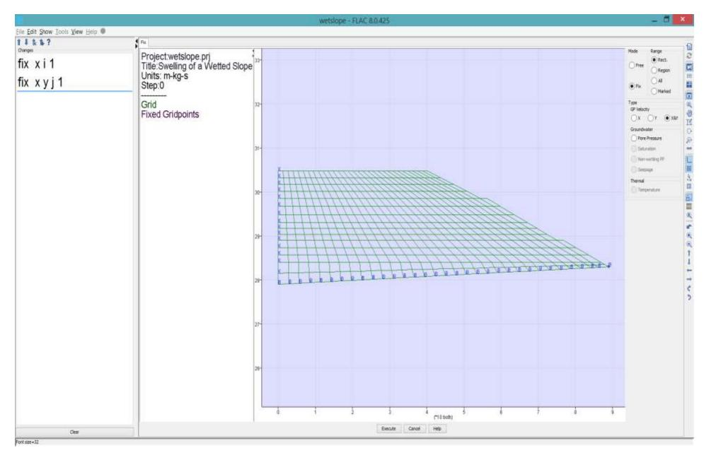
**Step 1-22** Enter [In Situ]/[Fix], select [Fix]/[X] and drag the mounse along the left boundary to fix the boundary in the x-direction. Select [Fix]/[X&Y] and drag the mouse along the bottom boundary to fix the boundary in both x- and y-directions.
