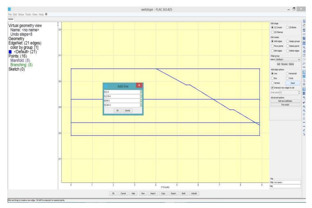
**Step 1-9** Create the line for the bottom boundary from x1=0.0, y1=279.0 to x2=89.0, y2=283.0
