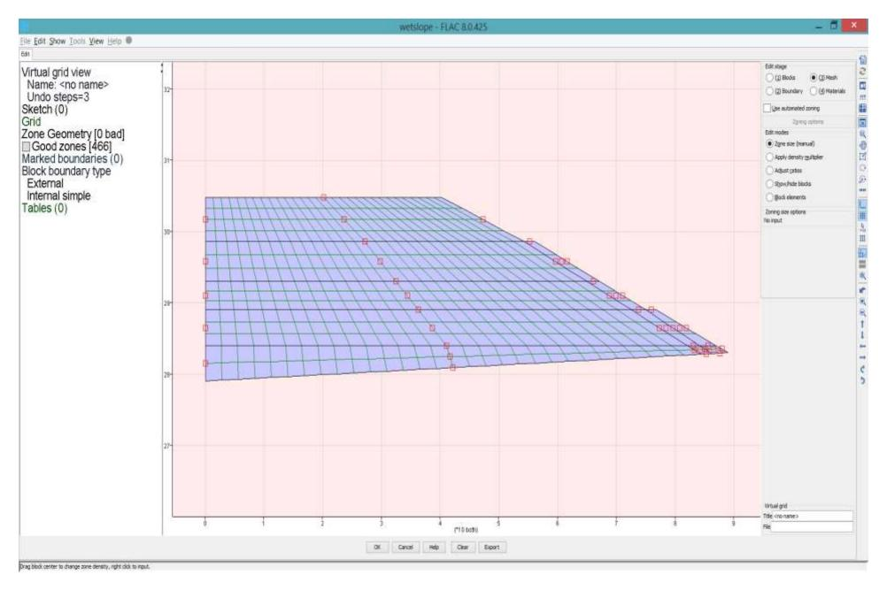
**Step 1-16** Press [Edit] to enter the Edit stage. Select the [Mesh] edit stage and manually divide the model into zoning as shown.
