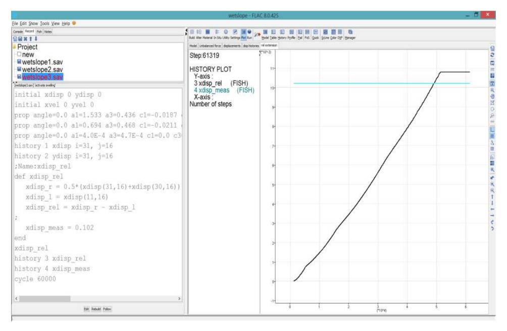
**Step 4-3** The relative extension (swelling motion) along the slope crest is calculated to be 108mm, and is compared to the measured value of 102mm in the history plot above.
