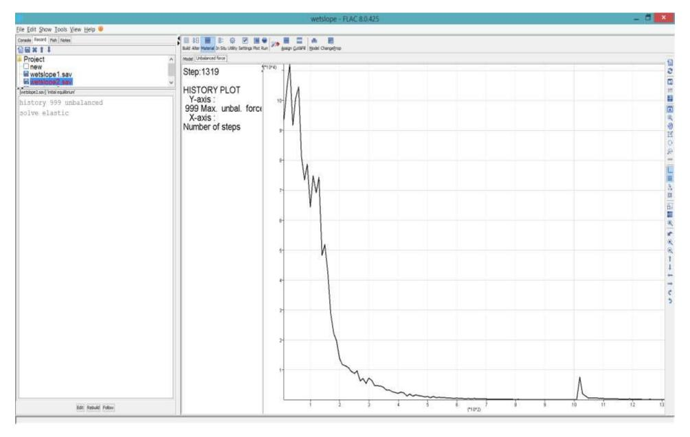
**Step 2-2** When the run stops, select [Plot]/[Quick] and [Unbalanced force] to plot the maximum unbalanced force history to check that equilibrium is reached.. Save the state as wetslope2.sav
