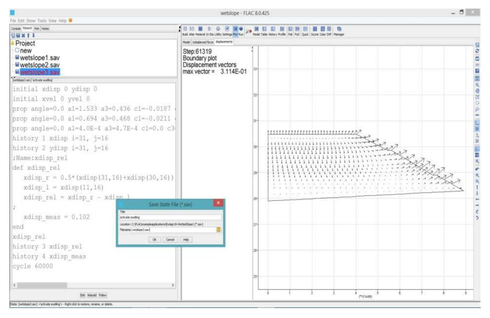
**Step 4-1** When the run stops, the swell motion is evaluated from a displacement vector plot. The state is saved as wetslope3.sav.
