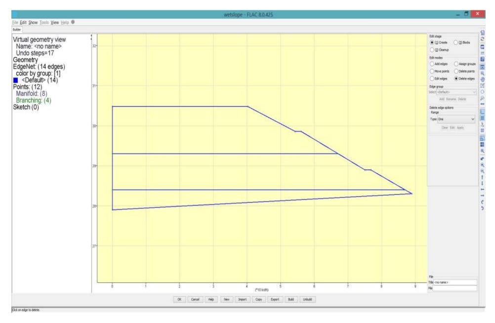
**Step 1-10** Select [Delete edges] to delete lines outside the slope.
