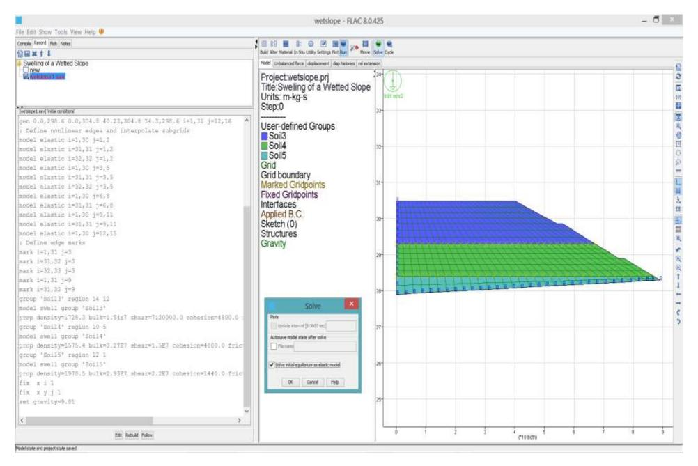
**Step 2-1** Select [Run]/[Solve], check [Solve initial equilibrium as elastic model] and press [OK] to calculate the initial stress state in the slope.
