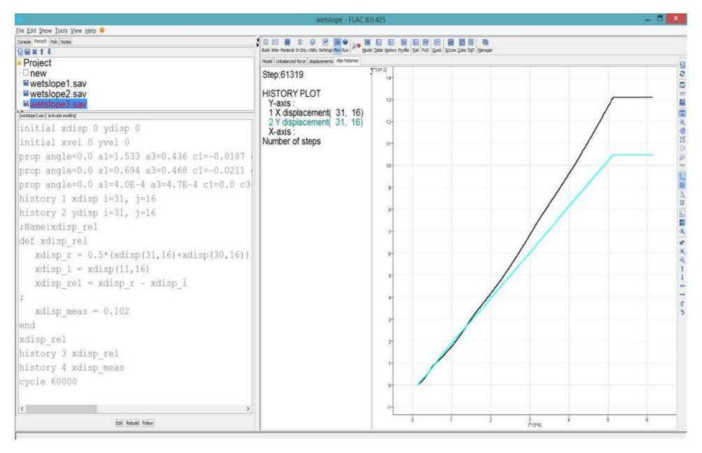
**Step 4-2** The horizontal movement at the slope crest is calculated to be 130.8mm and the vertical motion 104.5mm as noted from the x- and y-displacement history plots.
