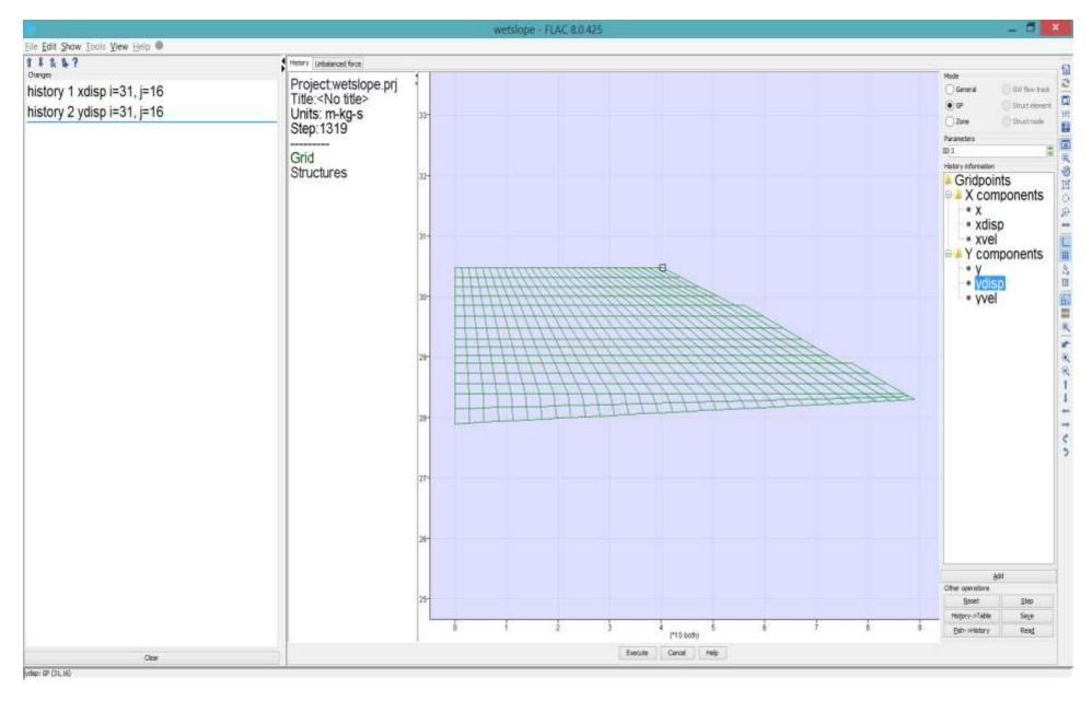
**Step 3-6** Monitor the x- and y-displacement at the slope crest in the [Utility]/[History] tool.
