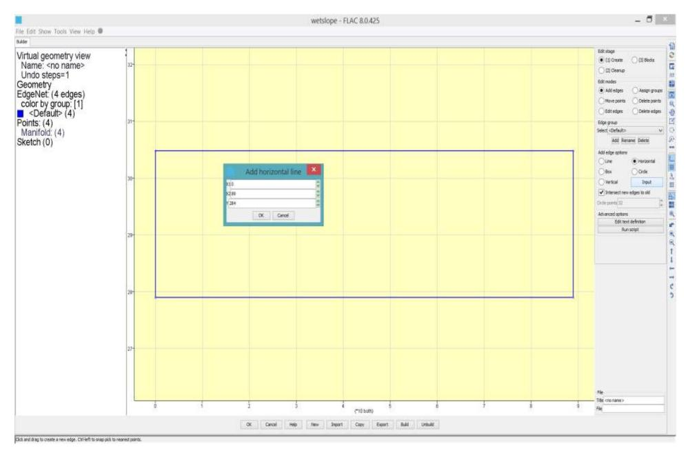
**Step 1-2** Select [Add edges]/[Horizontal] and locate a layer boundary at y = 284.0.
