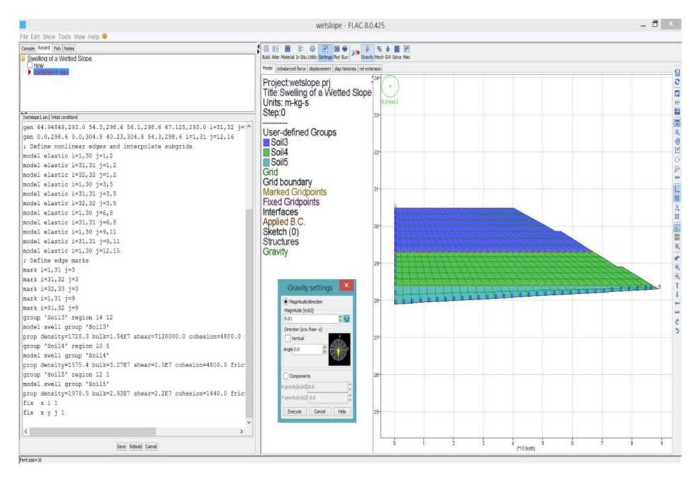
**Step 1-23** Select [Settings]/[Gravity] and assign gravitational loading.
