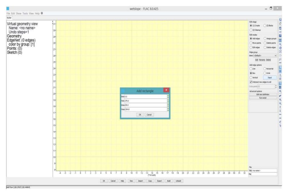
**Step 1-1** Enter the [Build]/[Generate]/[Geometry Builder] tool, select [Box] and set the outer dimensions at 0.0 < x < 89.0, 279.0 < y < 304.8.
