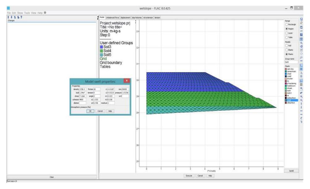
**Step 3-2** Enter the [Material]/[Model] tool, select [region] range, assign the group name **Soil3** and select the [swell] plastic model. Click on a zone inside the Soil3 region open the *Model swell properties* dialog. Enter all of the properties for **Soil3**.
