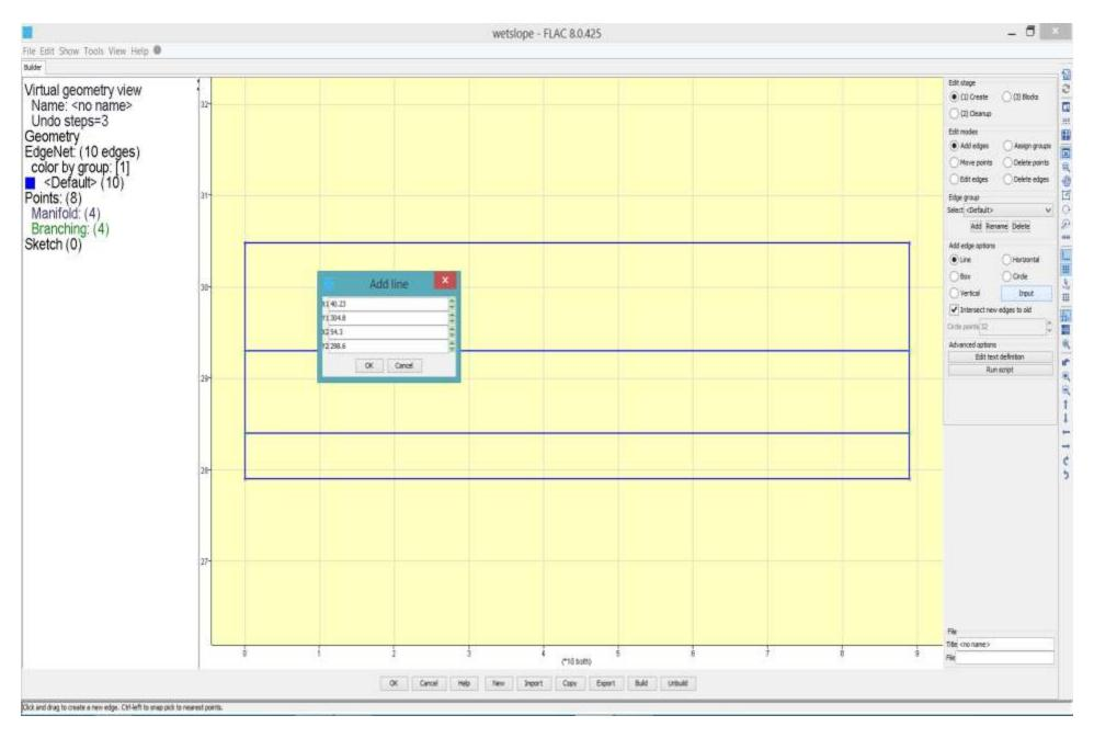
**Step 1-4** Select [Add edges]/[Line] to create the slope surface. Create the first line from x1=40.23, y1=308.8 to x2=54.3, y2=298.6.
