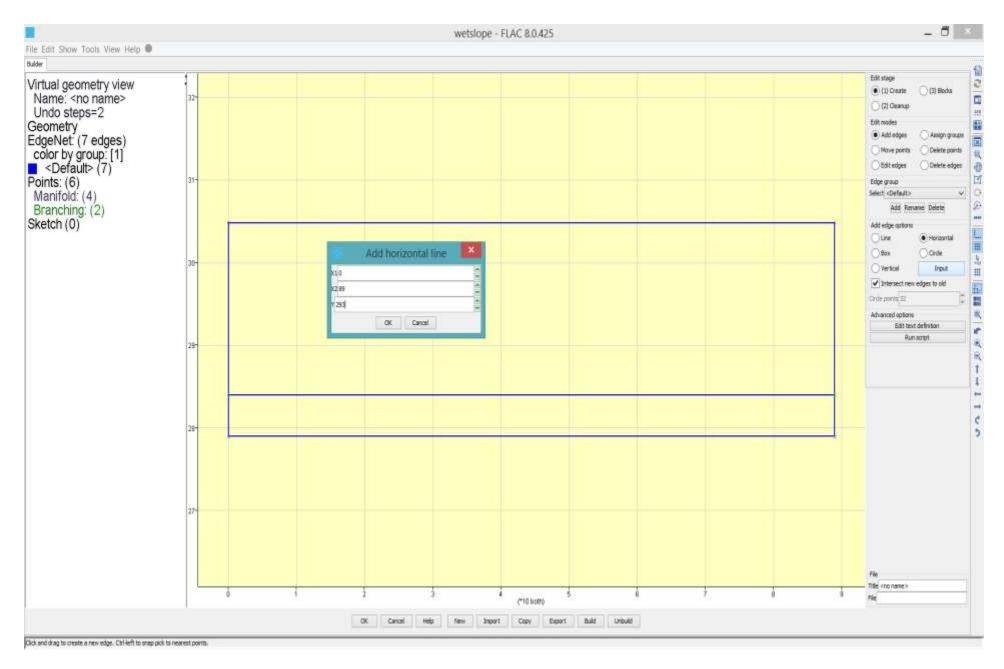
**Step 1-3** Select [Add edges]/[Horizontal] and locate a layer boundary at y = 293.0.
