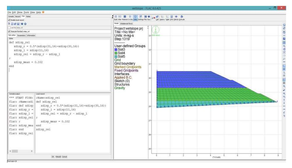
**Step 3-7** In the [FISH editor] pane, create a FISH function to monitor the relative motion at the crest between the midpoint of gridpoints i=31,j=16 and i=30,j=16 and gridpoint i=11,j=16. This relative horizontal movement corresponds to the location of the measured movement in the field. The measured movement (102mm) is defined by FISH variable, **xdisp meas**, for comparison to the calculated value.
