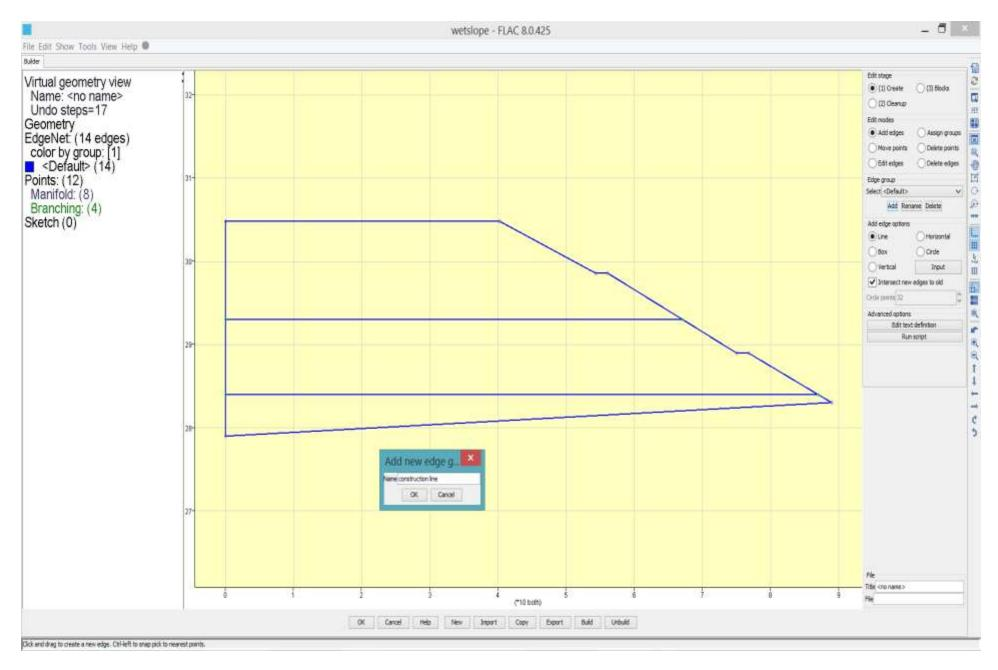
**Step 1-11** Create construction lines to divide the model into 4-sided blocks.
