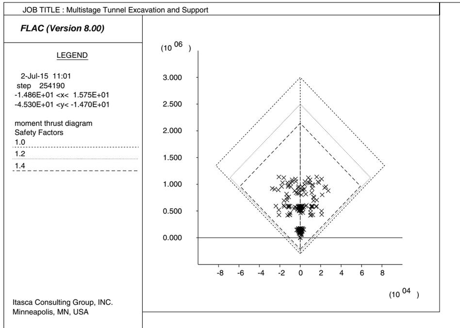
**Figure 11.11** *Moment-thrust diagram (tensile yield strength = 1 MPa, compressive yield strength = 10 MPa) for shotcrete liner at 100% relaxation at the last excavation stage*
