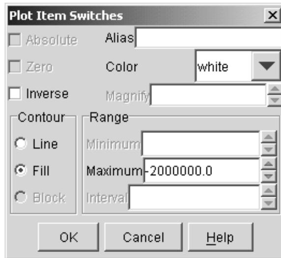
**Figure 11.8** *Plot Item Switches dialog; use the MAXIMUM switch to change the plot sense*
