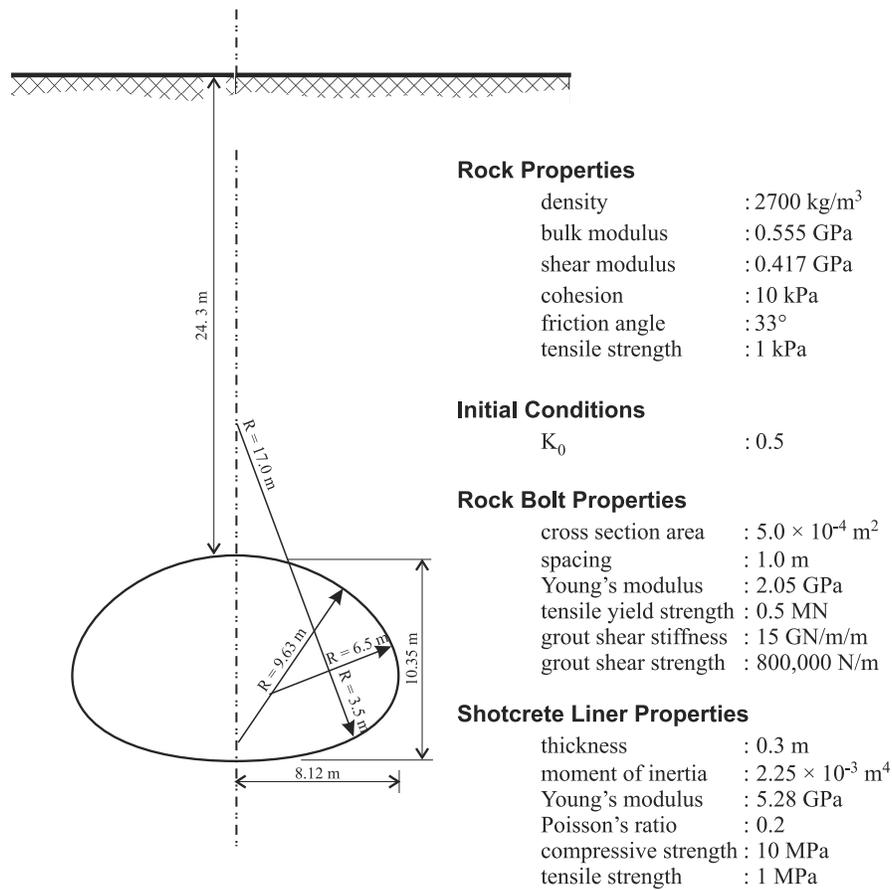
**Figure 11.1** Construction conditions for a multistage tunnel excavation and support
