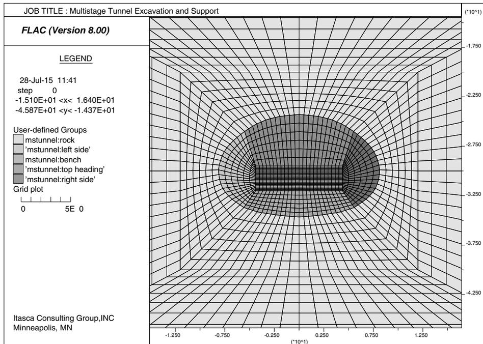
Figure 11.4 *Close-up of excavation stage groups for multistage tunnel construction*
