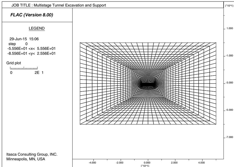
Figure 11.3 *FLAC grid for a multistage tunnel construction*
