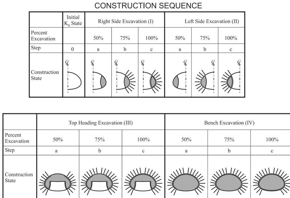
**Figure 11.2 Construction sequence for a multistage tunnel excavation and support**
