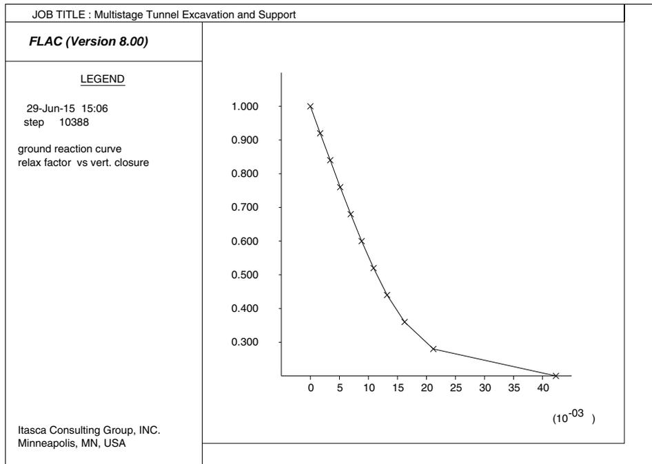
**Figure 11.5** Ground reaction curve: relaxation factor versus vertical closure
