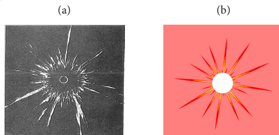
Figure 9. Fracture development around an explosively loaded borehole. (a) in a Plexiglas block 22 (b) numerical simulation
