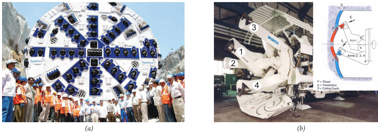
Figure 2. (a) Robbins TBM (Tunnel Boring Machine) for the 43.5-km long 10-m diameter water supply tunnel – AMR Project Andhra Pradesh, India 11 . (b) Wirth CMM (Continuous Mining Machine). 12
