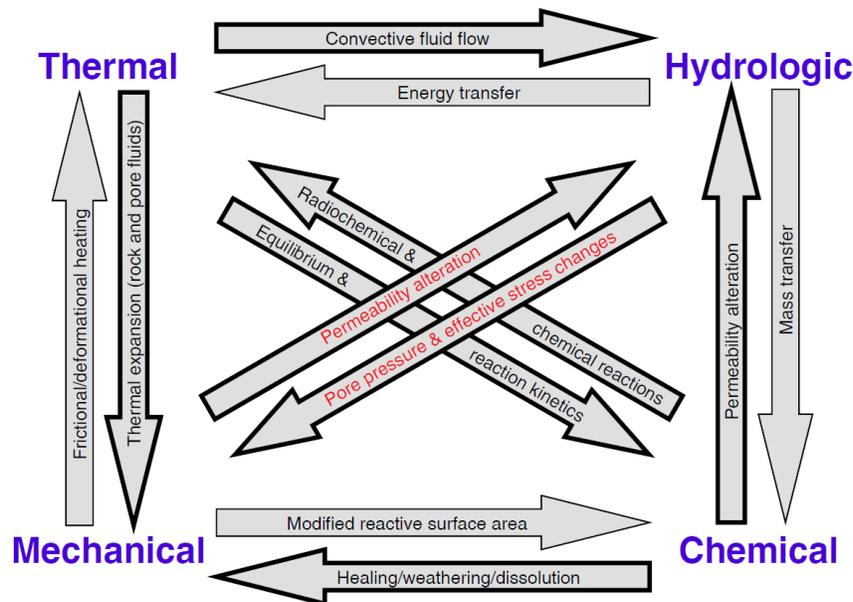
Figure 1. Coupled Thermo-Hydro –Mechanical- Chemical (THMC) processes in rock.
