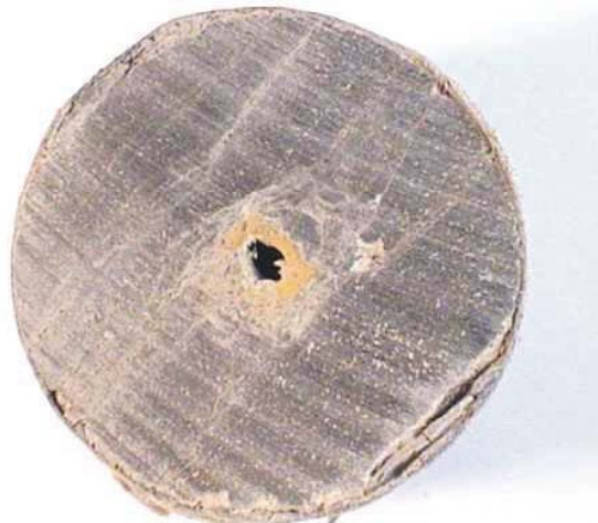
\sigma_c = 13 \text{ MPa} water circulated in inner borehole
