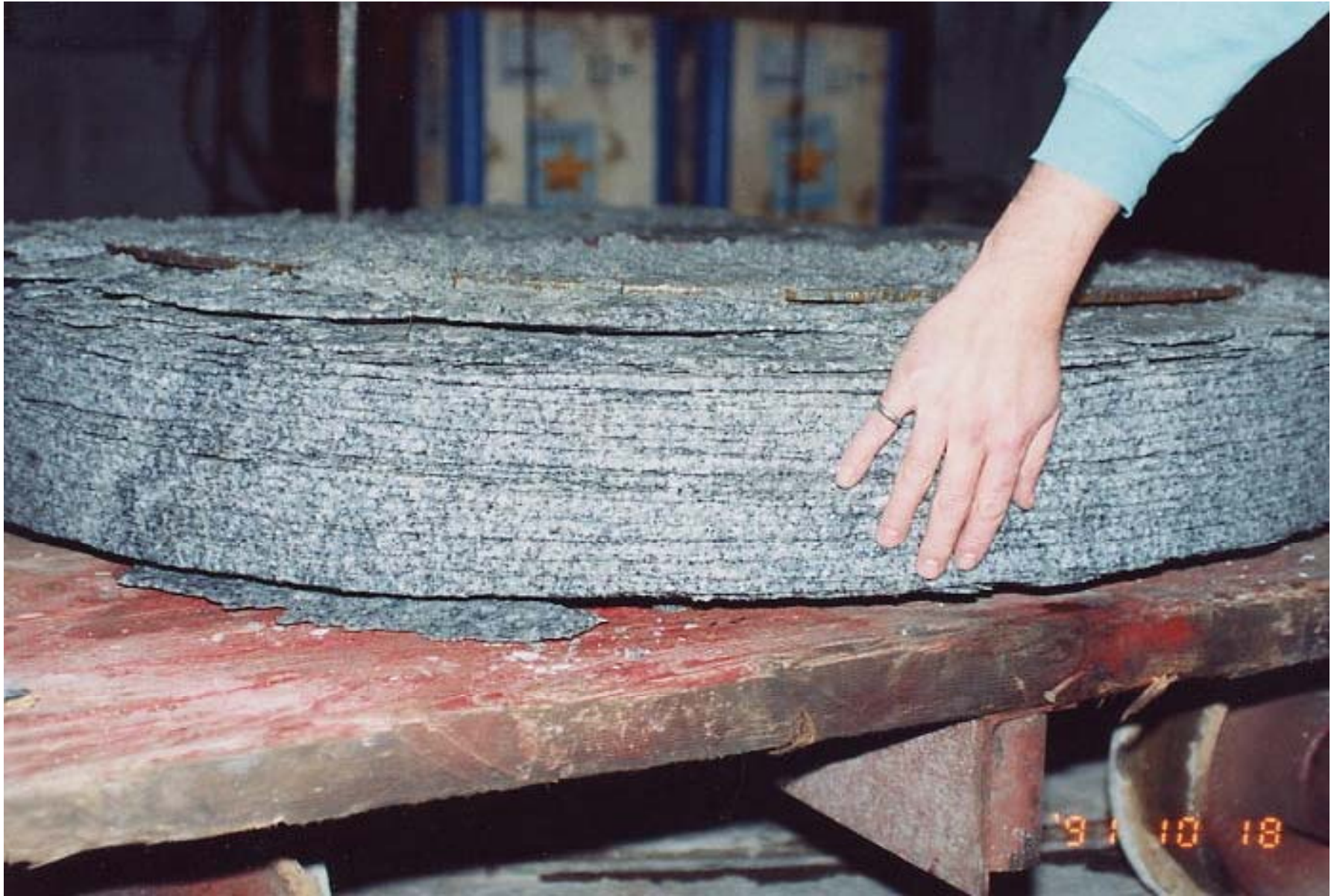
Discing of a 1.3 m diameter core from highly stressed rock (Courtesy of URL/AECL, Canada)
