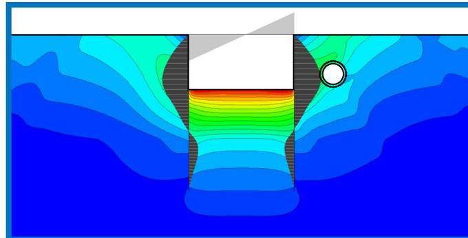
FLAC model of an excavation constructed in saturated ground. The excavation is dewatered during construction and is supported by diaphragm walls that are braced at the top by horizontal struts. Total displacement contours, wall moments, and strut horizontal displacements are shown.
