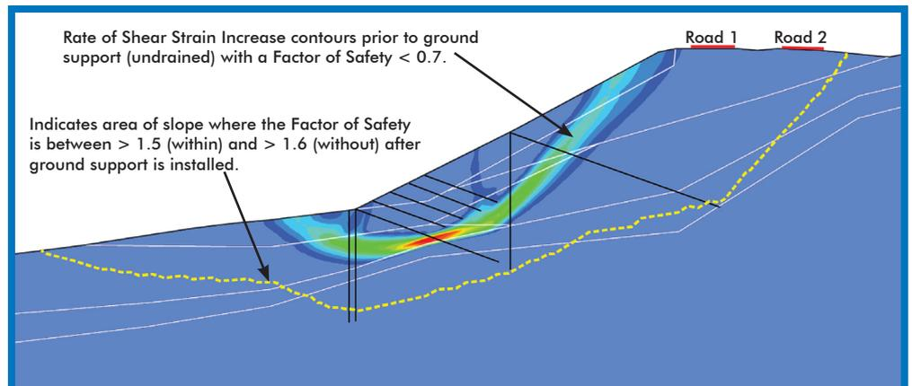
FLAC model results of a soil slope subjected to the load of two new highways (red lines) near the crest before and after a ground support design is installed. Different soil materials are delineated by the solid white lines and the ground support is represented by black lines. The final support design consisted of a combination of drilled shafts, pre-tensioned grouted anchors, and fiberglass soil nails.
