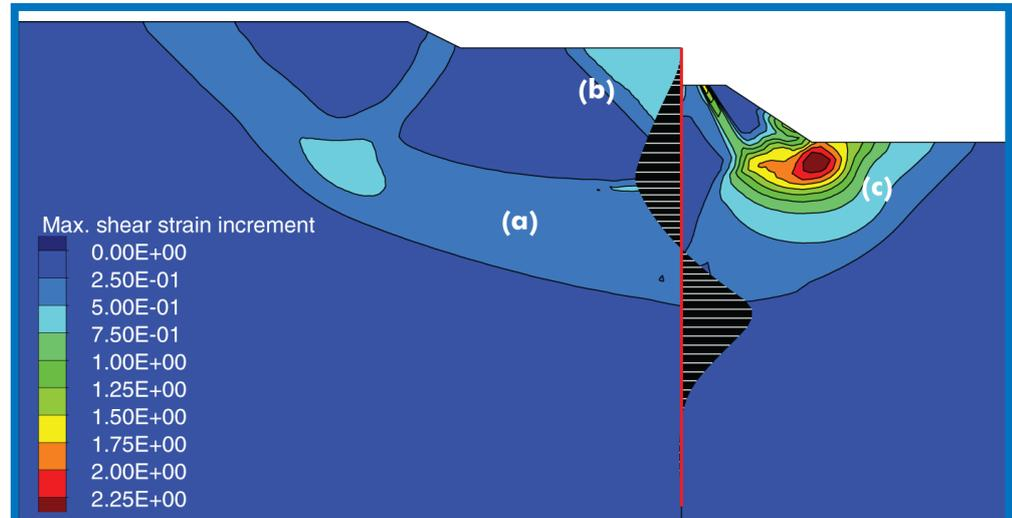
▲ *FLAC* is capable of modeling multiple physical failure mechanisms as they evolve naturally. In this example, a slope is reinforced with a sheet pile wall (SPW), shown in red. A factor of safety less than 1 is determined due to (a) global deep seated shear failure, (b) an active wedge behind the SPW, and (c) the bearing capacity of the lower-most slope toe. The bending moments of the SPW are also shown in black.
