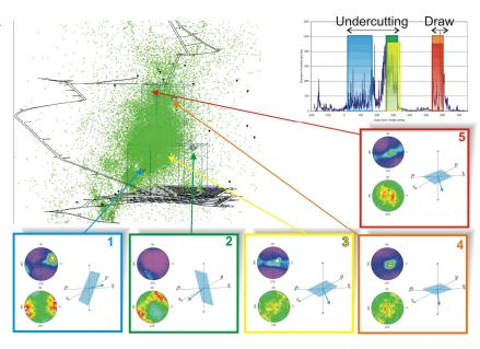
SRMs from each domain underwent tests resulting in the sample exhibiting over 100,000 cracks each. Statistical methods were applied to compare the fractures inferred from seismicity in the mine and those predicted by the SRM as a way of validating the predictive capabilities of SRM tests.
