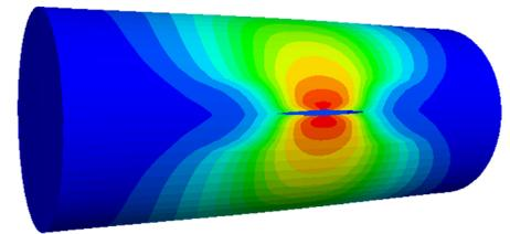
Displacement magnitude contours for a longitudinal fracture.
