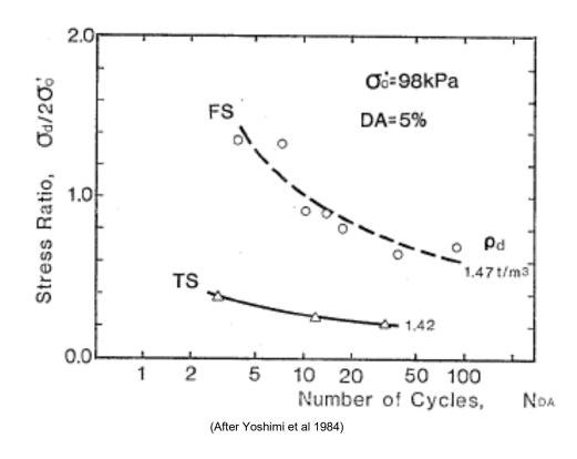
Yoshimi et la (1984) showed that undrained cyclic strength of **triple-tube samples** was ~30%, and **reconstituted samples** was 30~60%, of that of **frozen samples** (supposed close to field conditions).
