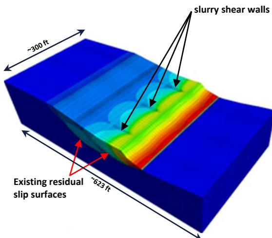
FLAC3D model showing ground displacement contours for one case includes three slurry shear walls and two slip surfaces.
